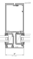
Factory-assembled and factory-glazed under controlled conditions
