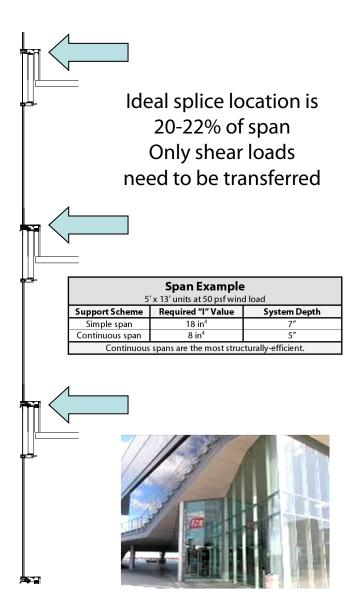
The **ideal splice location** is typically 20% to 22% of span, occurring at the "zero moment" point, where flexural stresses reverse from compression to tension at mullion flanges.
