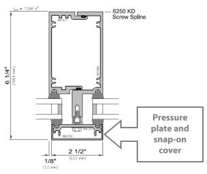
"pressure wall," because exterior extruded aluminum plates are screwapplied to compress glass between interior and exterior bedding gaskets. A snap-on cover or "beauty cap" is then used to conceal fasteners.
