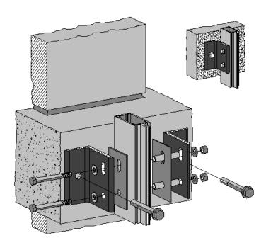
Three-way adjustment is critical. Can be bolted or welded in place In one standard anchorage method, "double angle" mullion anchors straddle both sides of the vertical mullion, and are secured with a throughbolt and pipe spacer.
